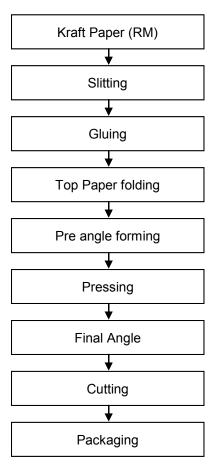
Corner boards manufactured by us are through a single line process done on a continuous basis. The process flow involved in manufacturing of the corner board is explained hereunder:
