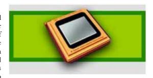
one pixel in a projected image. When a DMD chip is coordinated with a digital video or graphic signal, a light source, and a projection lens, its mirrors can reflect an all-digital image onto a screen or other surface. The DMD and the sophisticated electronics that surround it are what we call Digital Light Processing technology.
